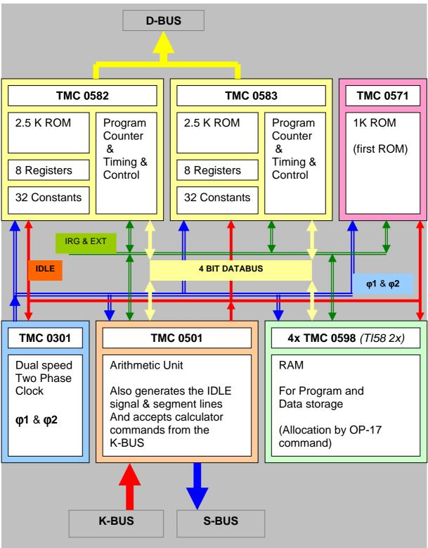
Based on the above diagram we may conclude there are two sets of signal-busses in the TI59.
